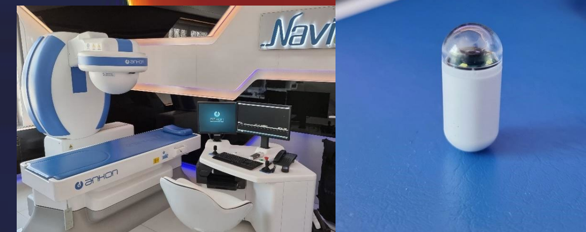
Fig. 1: Magnetically controlled capsule endoscopy work station (left) and magnetic capsule endoscope (right)
